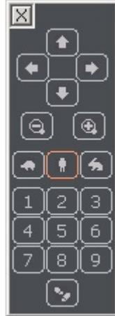
The arrows indicate directions, zoom in and zoom out options are located underneath. The turtle, man and rabbit icons determine the speed of the camera movement after an arrow is pressed. More precisely, that means that when you press an arrow, the dome will be moved by a specified interval. If the turtle icon is selected, the dome will move very slowly, the human icon causes the dome to move at medium speed and pressing the hare icon results in very fast movement of the dome.
