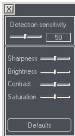
The **Detection sensitivity** parameter relates to the sensitivity of motion search in a given archive for a specified camera. Move the indicator to the right in order to increase the sensitivity.
