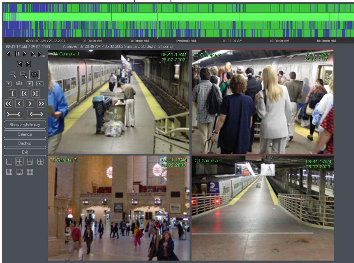
The upper part of the archive window displays a time chart of the recordings; the **log**. The green bars represent recorded camera images. Use the mouse pointer to select a particular position in the log, to display the image recorded at that moment.
