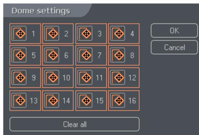
Click the camera icons in order to specify, which camera dome control the user will have access to. The domes that can be controlled by the user are highlighted with an orange border.
