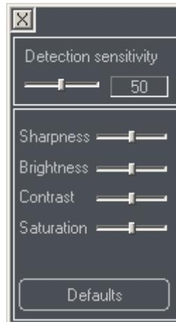
The **Detection sensitivity** parameter concerns the sensitivity of searching for motion in the archive for a given camera. Move the indicator to the right in order to increase the sensitivity.
