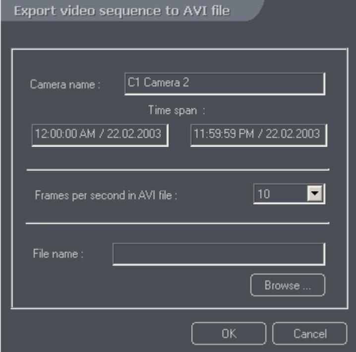
First, select the camera to export video from, time span, fps rate and the file name. After clicking **OK** button you have to select the codec to encode the file.
