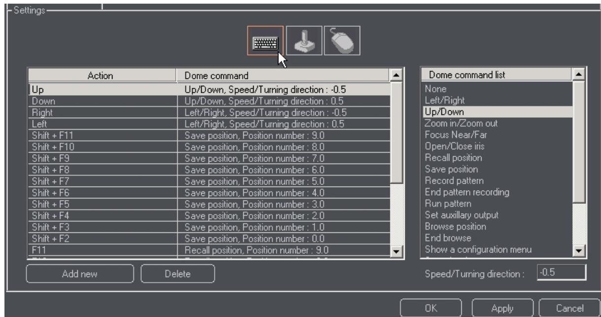
When you select the keyboard, different keys can be bound to different functions (double-click an item, or press the **Add new** button, if there are no items). Press a key on the keyboard and select a function for this key on the right, e.g. **Set position**, **Turn left**, **Turn right**. You can assign unlimited number of commands. Set the speed of rotation in range from  $-1$  to  $+1$ .
