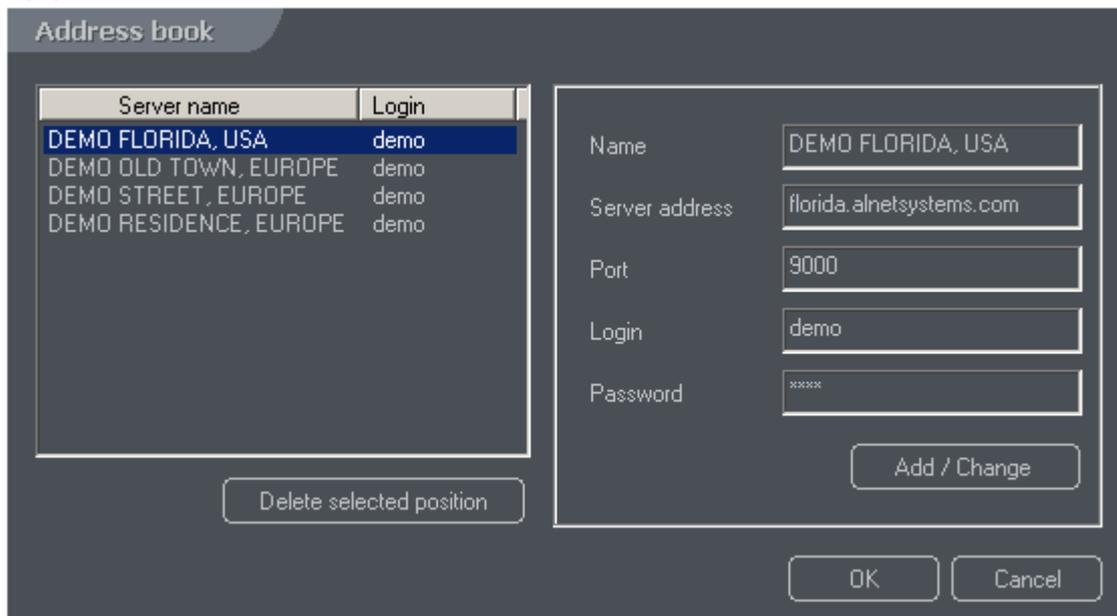
In order to configure settings for a new server, press the **Add/Change** button and enter the name (**Video Server** by default). Specify the Internet address of the computer or its **IP** number, **port** number (9000 by default), login and password, and confirm.
