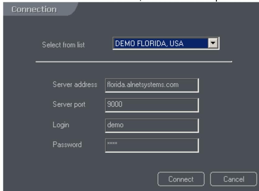
A new small window with messages concerning the connection process will appear on the screen. After a while (maximum 1 minute) the cameras, alarm inputs and output switches should appear, but only the ones that the user has rights to (set in the server configuration).
