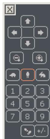
The arrows indicate directions, zoom in and zoom out options are located underneath. The turtle, man and rabbit icons determine the speed of the camera movement after an arrow is pressed. More precisely, that means that when you press an arrow, the dome will be moved by a specified interval. If the turtle icon is selected,
