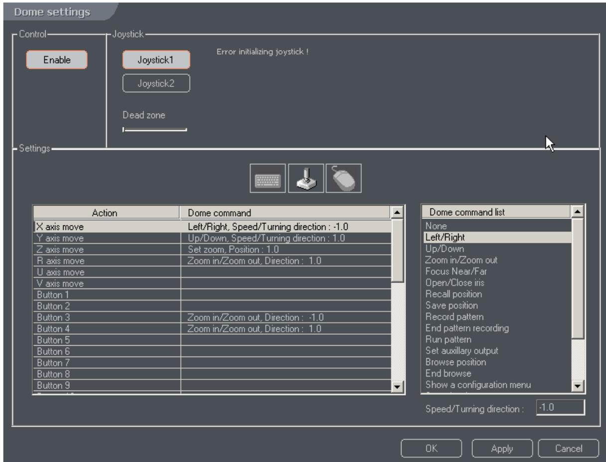
After the window is opened, select the USB joystick (at present only one joystick is supported) and select the protocol according to the type of dome to be controlled: Lilin, Sensormatic, Pelco. Next, select the serial port, to which the RS-485 converter is connected (COM1 or COM2).
